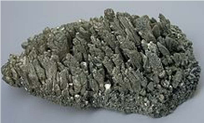
Vapor-deposited magnesium crystals from the Pidgeon process
