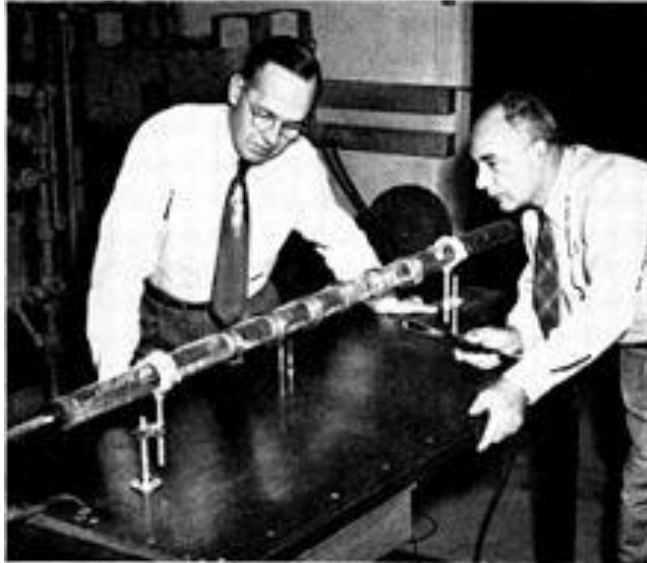
(left) Pfann, at left, showing the first zone refining tube, Bell Labs, 1953
